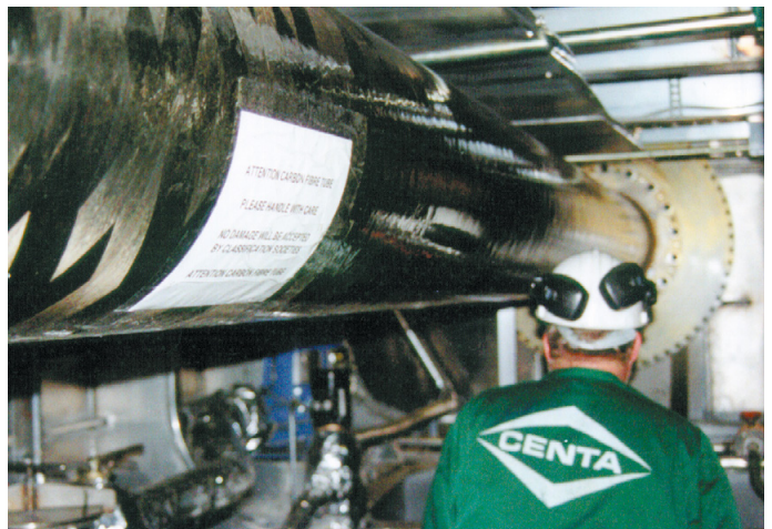
CENTADISC carbon fibre shaft in »Jumbo Cat«.
